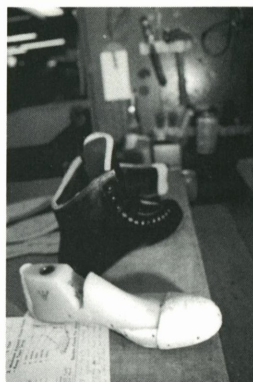
Skates are built on a plastic foot mold, called a last. Lasts give consistent foot dimensions for skate sizes, fits and styles.
