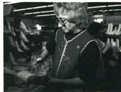
In the final stages of production, a worker cleans, hand-polishes, inspects and gives the boots a top spray for shine.
